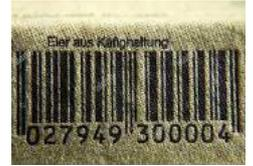
**7** Distortion due to the location on the packaging – on a curved structure a vertical placement is better.
